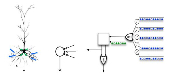
The image above shows a picture of a biological neuron on the left, a simple artificial neuron in the middle, and an HTM neuron or "cell" on the right. The purpose of this appendix is to provide a better understanding of HTM cells and how they work by comparing them to real neurons and simpler artificial neurons.
