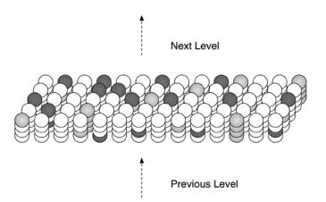
Figure 2.3: At any point in time, some cells in an HTM region will be active due to feed-forward input (shown in light gray). Other cells that receive lateral input from active cells will be in a predictive state (shown in dark gray).
