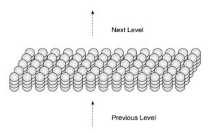
Figure 1.3: A section of an HTM region. HTM regions are comprised of many cells. The cells are organized in a two dimensional array of columns. This figure shows a small section of an HTM region with four cells per column. Each column connects to a subset of the input and each cell connects to other cells in the region (connections not shown). Note that this HTM region, including its columnar structure, is equivalent to one layer of neurons in a neocortical region.
