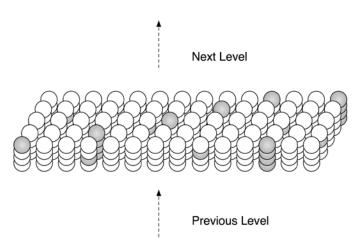
Figure 2.2: By activating a subset of cells in each column, an HTM region can represent the same input in many different contexts. Columns only activate predicted cells. Columns with no predicted cells activate all the cells in the column. The figure shows some columns with one cell active and some columns with all cells active.
